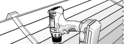
Drill 4 holes in DET 2, diam. 10mm
