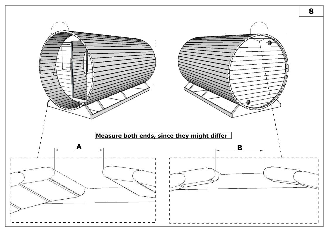
NB! Connect the points A-A and B-B before cutting
