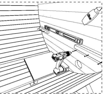
Use glue between supporting beam and wall
