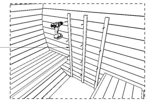
NB! Electrical heaters do not require DET L. Mount DET 13 directly to the wall using 3x40 screws in case of the electrical heater
