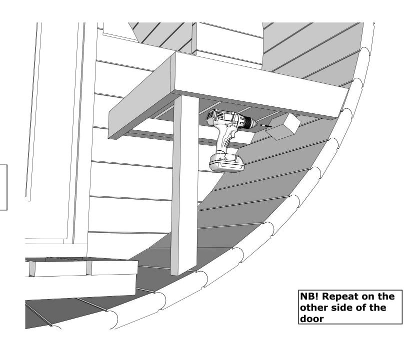
NB! Drill a 4mm hole before fixing DET 11 with a screw NB! Use small nails to install roof shingles. Also use the roof shingles manual for reference how to install the shingles properly
