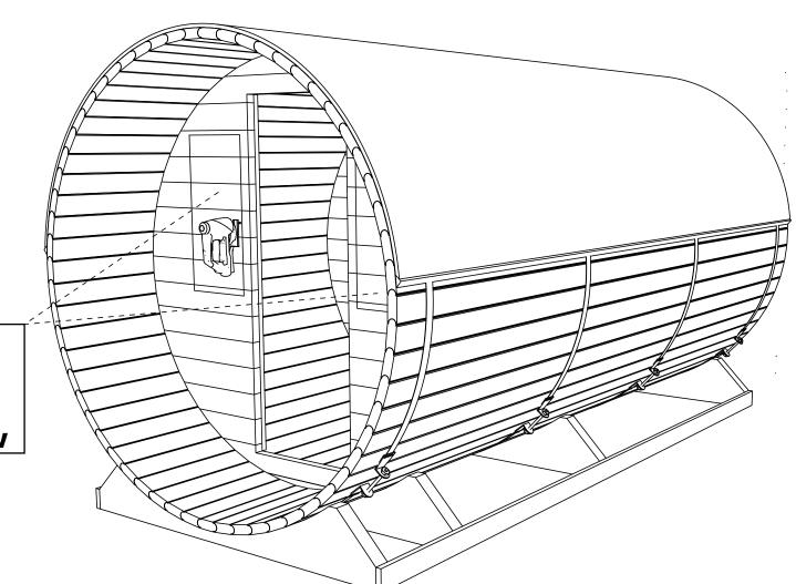
Cut out windows following the guidelines using a circular or jig saw
