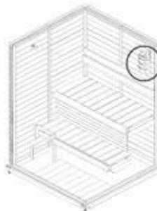
The wall has a pre-drilled hole(s) for the lights. Insert wire(s) to the conduit(s) provided for the lights.
